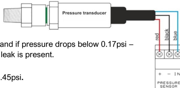
The sensor will monitor the gas supply pressure and if pressure drops below 0.17psi – the gas valve will close as this could mean a gas leak is present.
